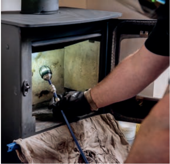
Thanks to the LEDs in the camera head, you can see even in the darkest places.
